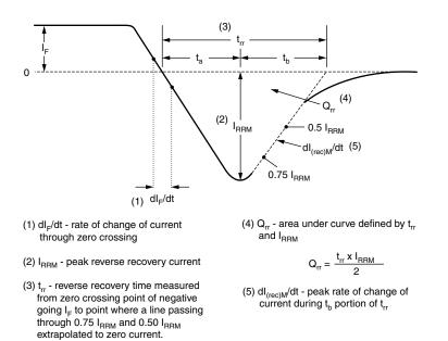
Fig. 10 - Reverse Recovery Waveform and Definitions
