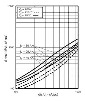
Fig. 8 - Typical  $dI_{(rec)M}/dt vs. dI_F/dt$
