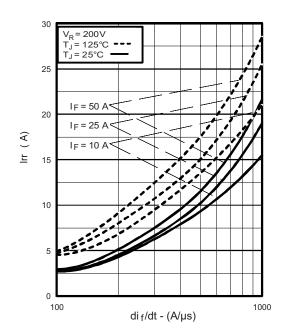
Fig. 6 - Typical Recovery Current vs. dI<sub>F</sub>/dt
